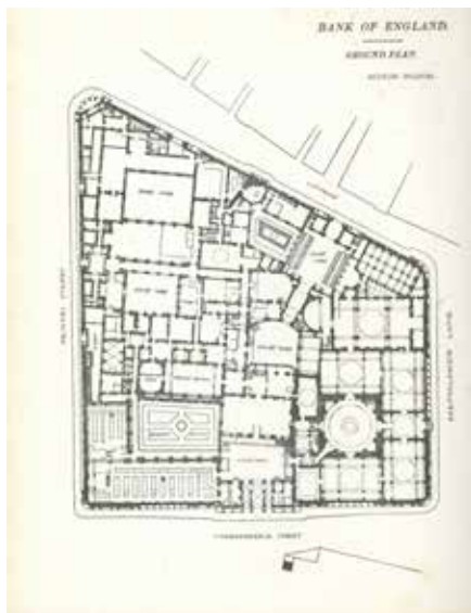
Ground plan of the Bank before the rebuilding in the 1920s. The churchyard of St Christopher Le Stocks can be seen on the left hand side, named as 'garden court'. Bank of England Archive, Ref. E8/7.
